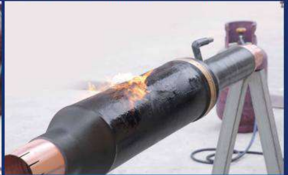
非阻燃型：燃烧后火焰不会自熄，有滴落物 Non-flame retardant type: the flame will not self-extinguish after burning, and there are dripping objects.
